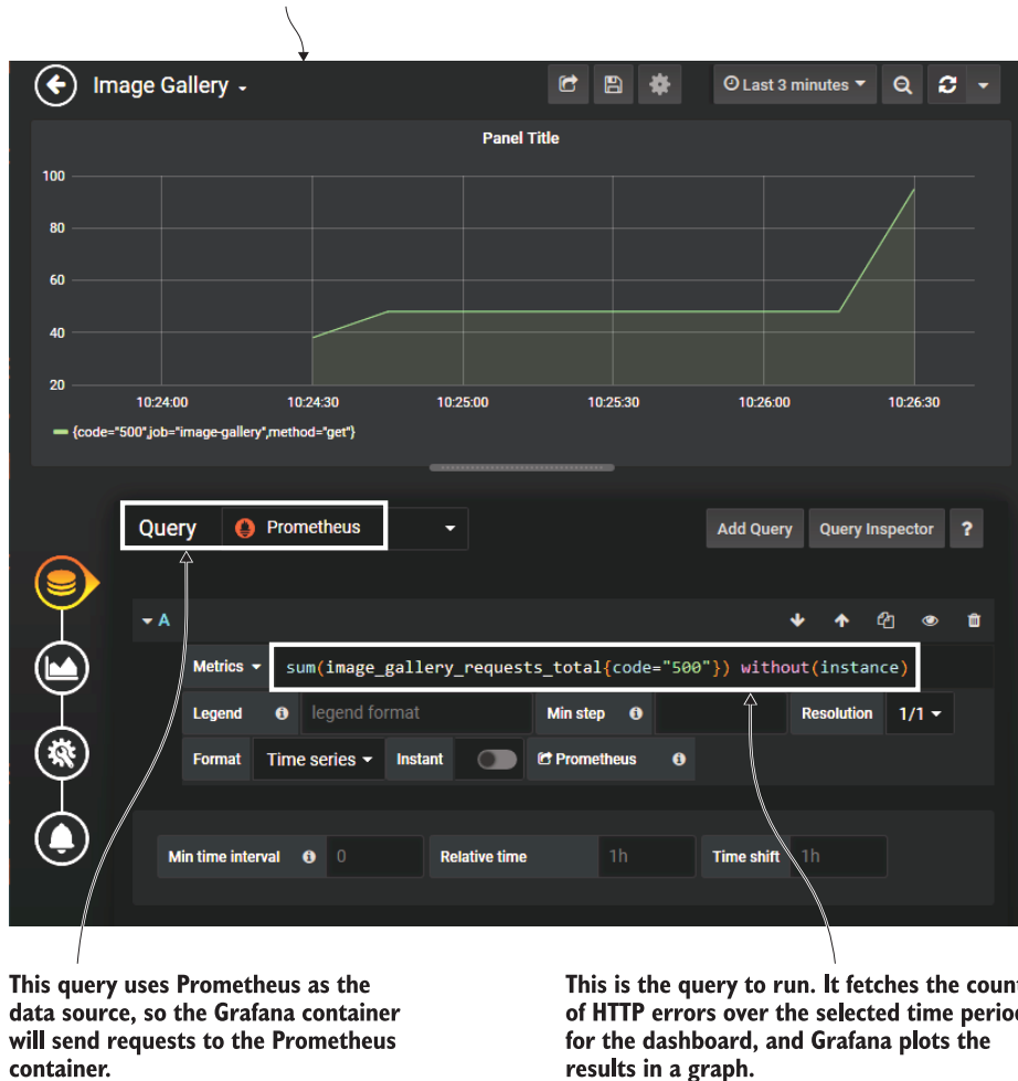
Figure 9.16 Adding a new panel to the Grafana dashboard to show HTTP errors
