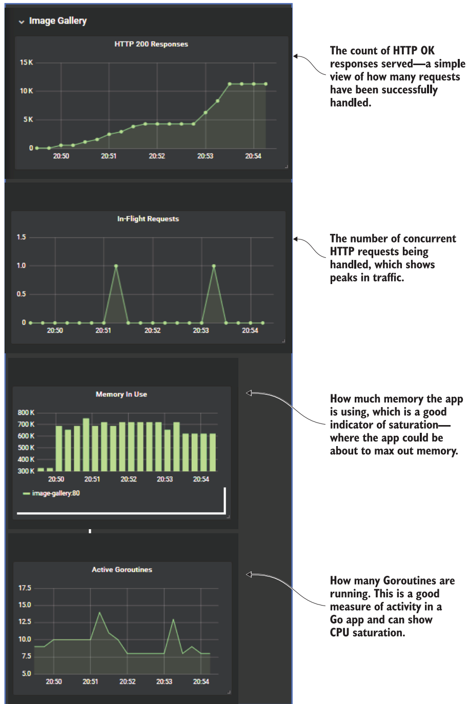
Figure 9.14 A closer look at the application dashboard and how visualizations relate to the golden signals
